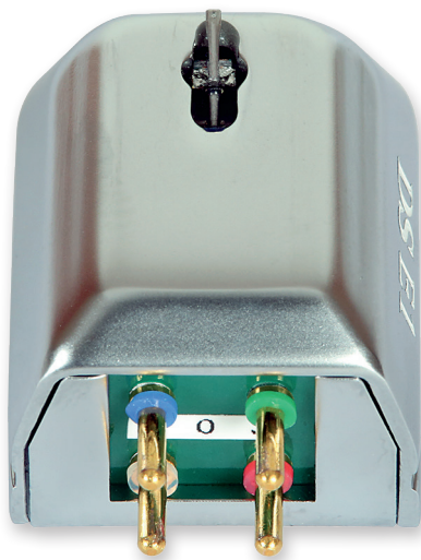
ABOVE: The DS-E1's pins are clearly marked and separated. Just visible is the alloy cantilever, tie-wire suspension and elliptical stylus [see also p54]
